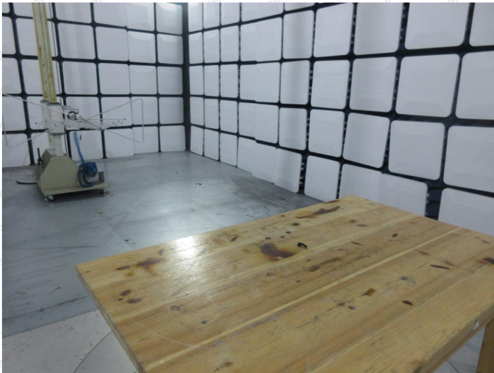
Photo of Radiation Emission Test
