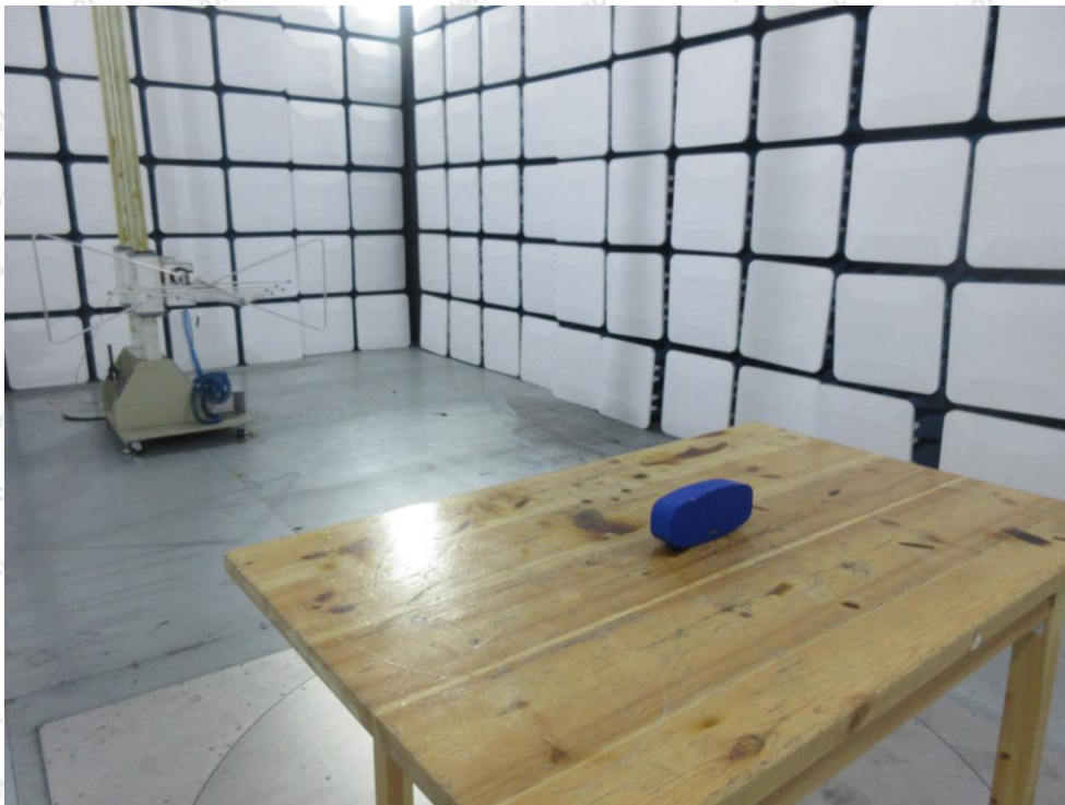
Photo of Radiation Emission Test
