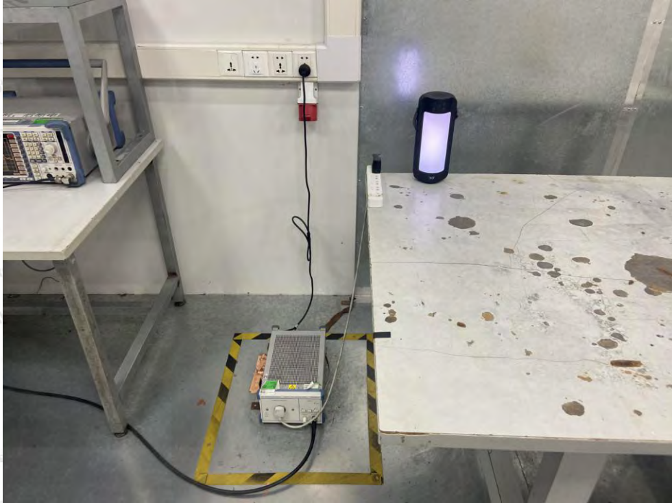
Photo of Power Line Conducted Emission Test
