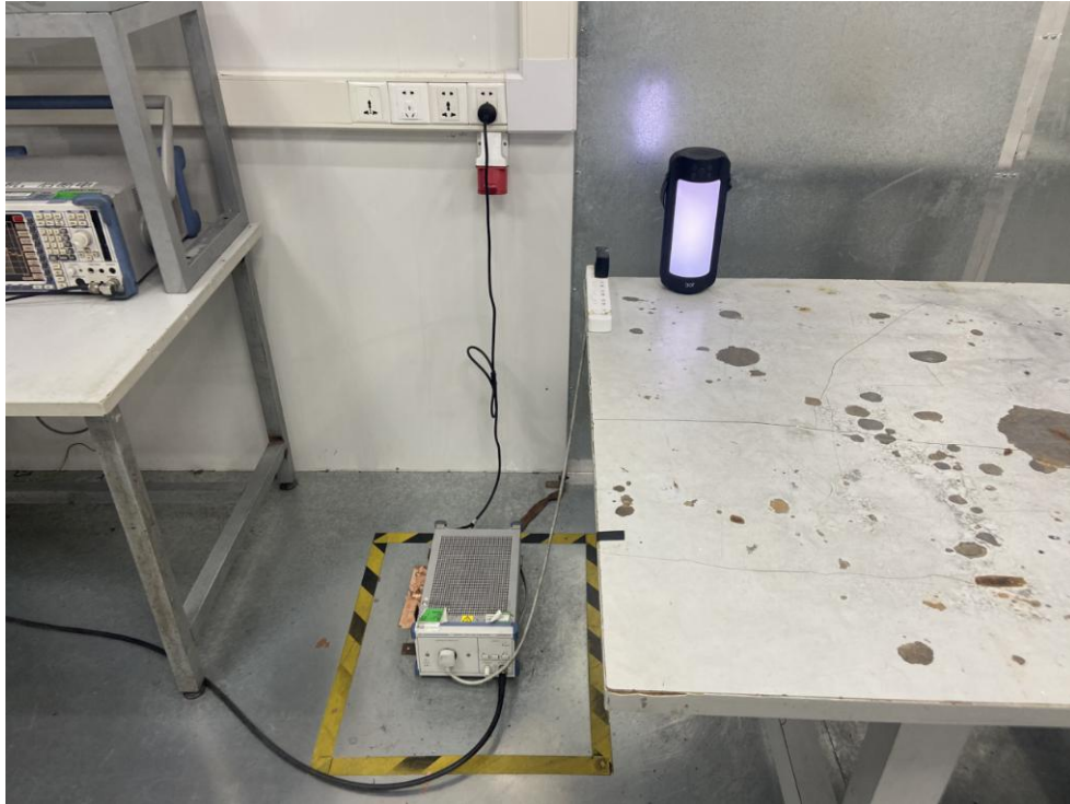
Photo of Power Line Conducted Emission Test
