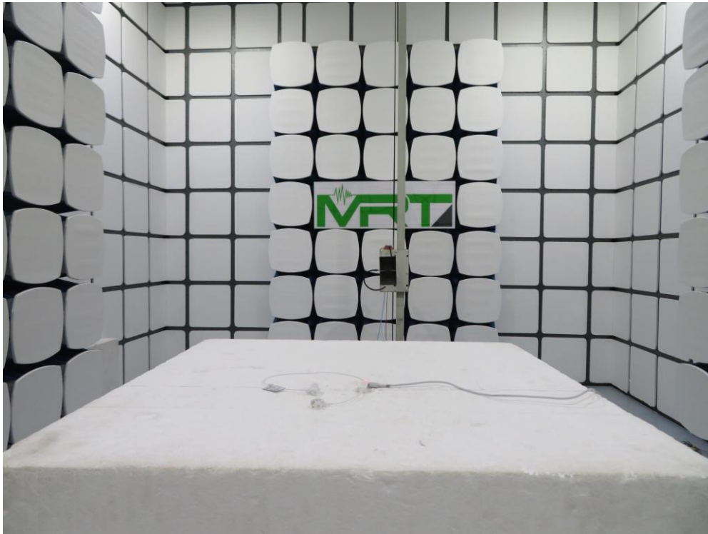
Description: Radiated Spurious Emission Test Setup for 18GHz ~ 25GHz
