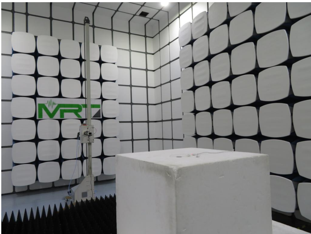
Description: Radiated Spurious Emission Test Setup for 18GHz ~ 25GHz
