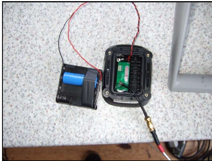
Photo 1 Connection to Antenna and battery during conducted power measurements.
