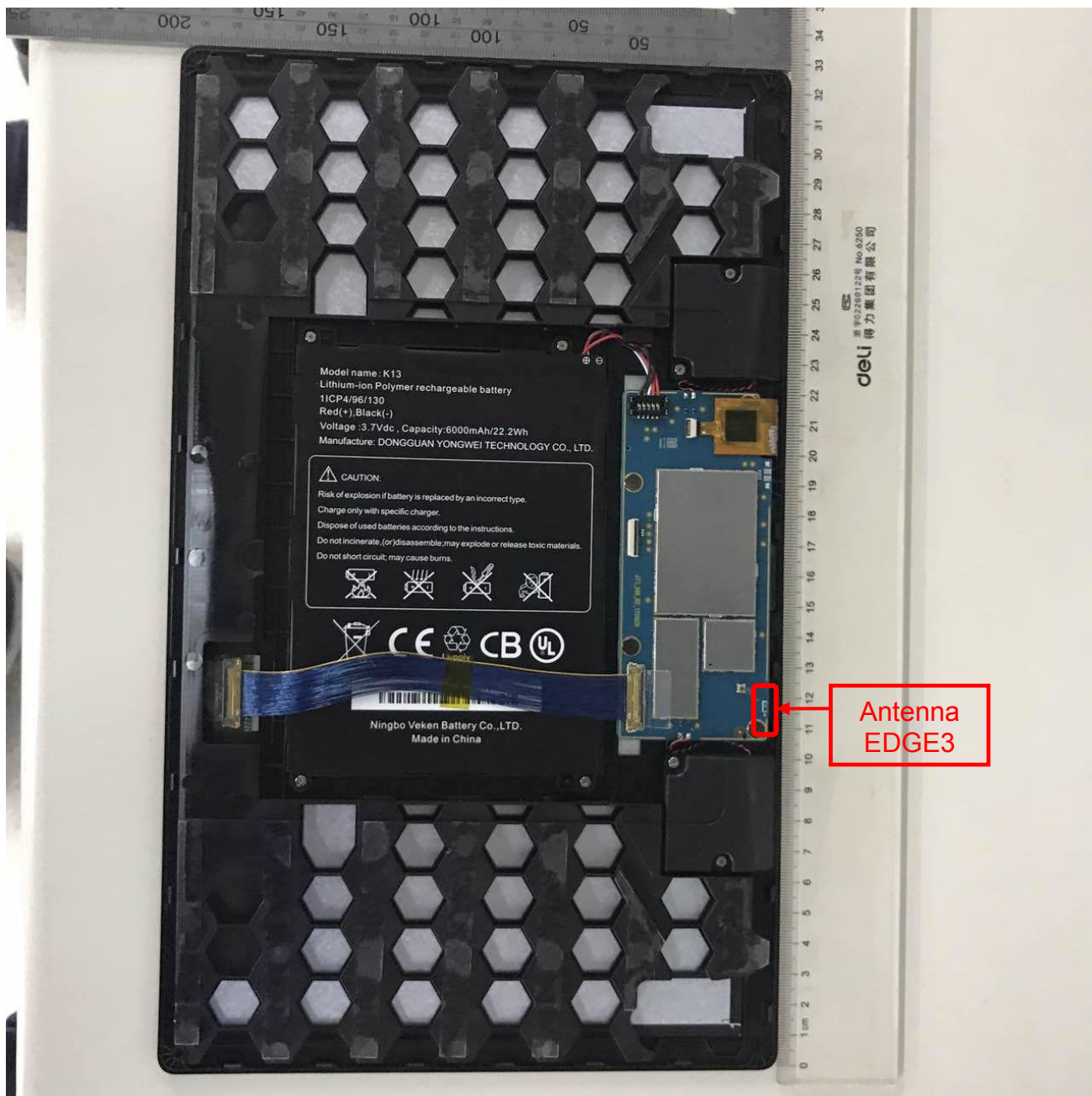
Antenna Locations & Separation Distances
