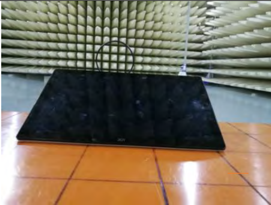
Spurious Radiated Emissions Test setup (below 30MHz)
