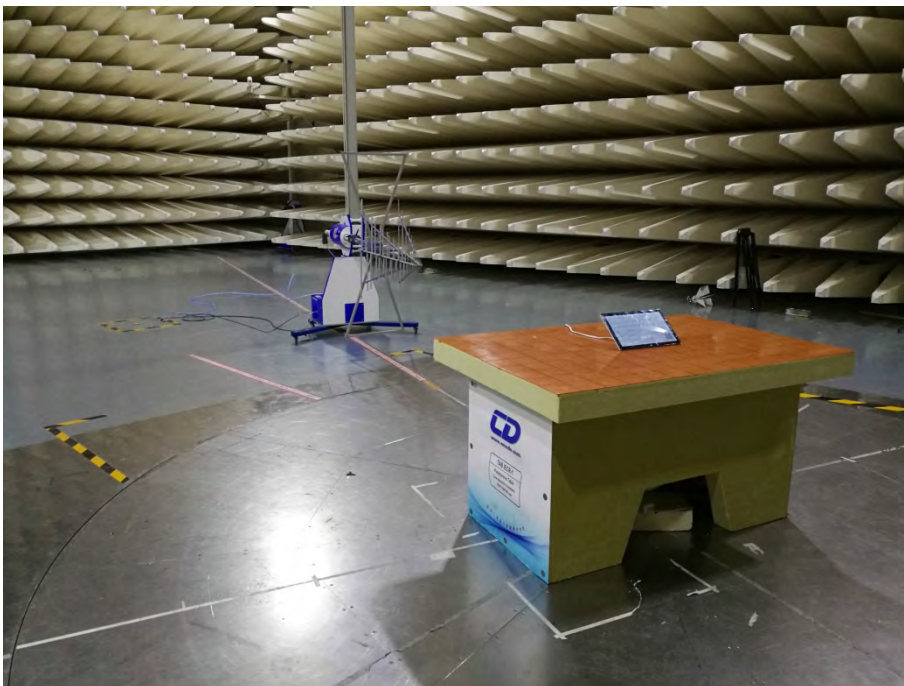
Spurious Radiated Emissions Test setup (30MHz~1GHz)
