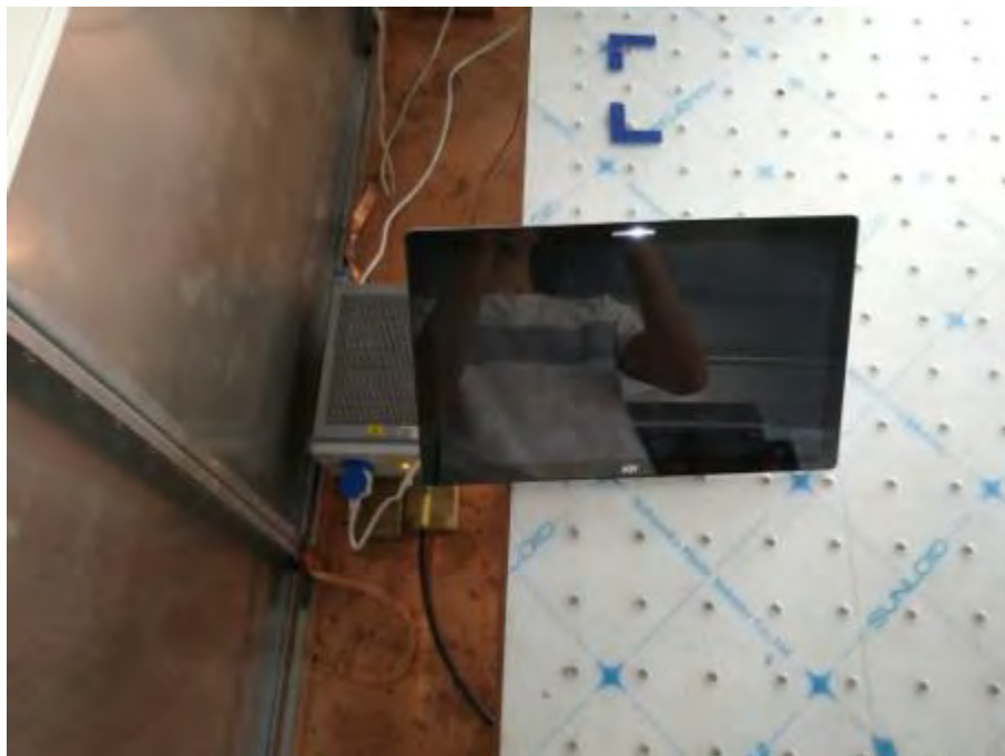
Conducted Emissions Test Setup (with charger)
