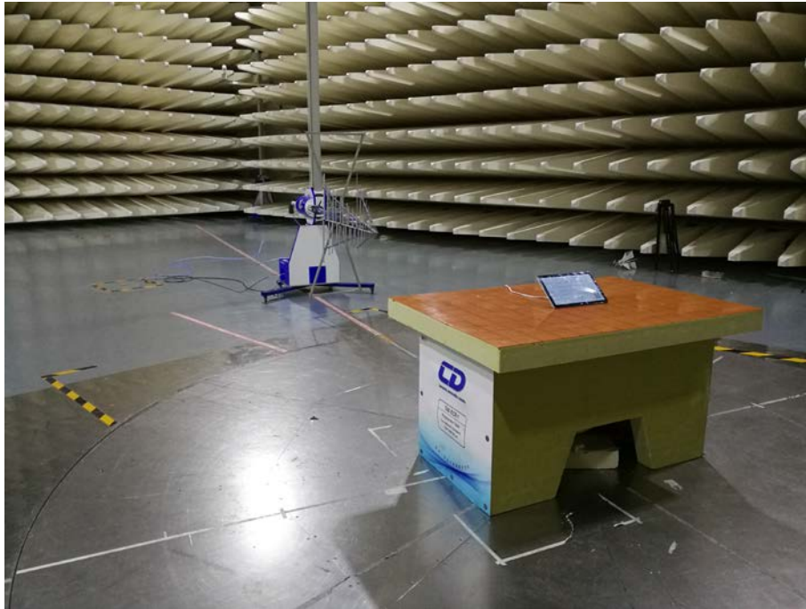
Spurious Radiated Emissions Test setup (30MHz~1GHz)
