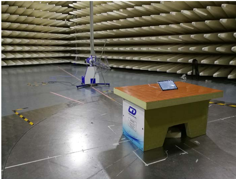
Spurious Radiated Emissions Test setup (30MHz~1GHz)
