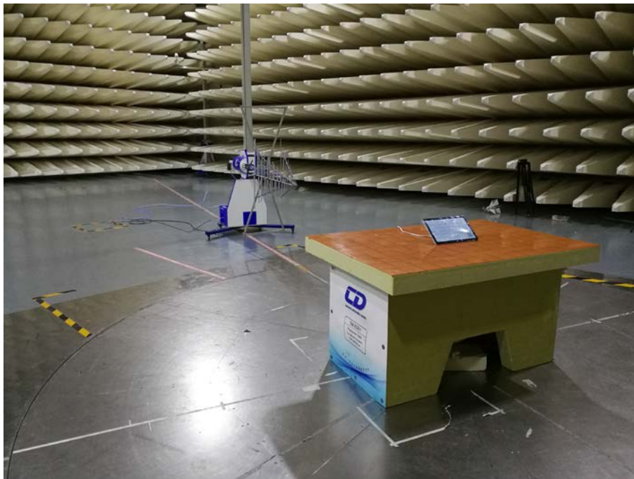
Spurious Radiated Emissions Test setup (30MHz~1GHz)
