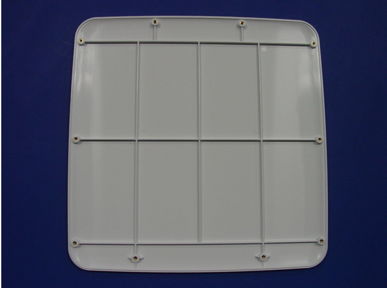
Back of Radome
