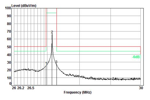
Condition: 3m HORIZONTAL Job No. : 06068CR Test mode: a
