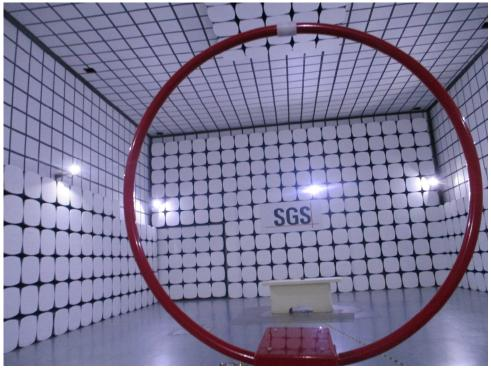
8.2 Radiated Emissions(30MHz-1GHz) Test Setup
