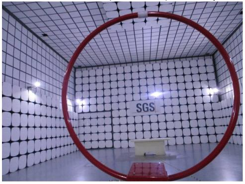
1.2 Radiated Emissions(30MHz-1GHz) Test Setup
