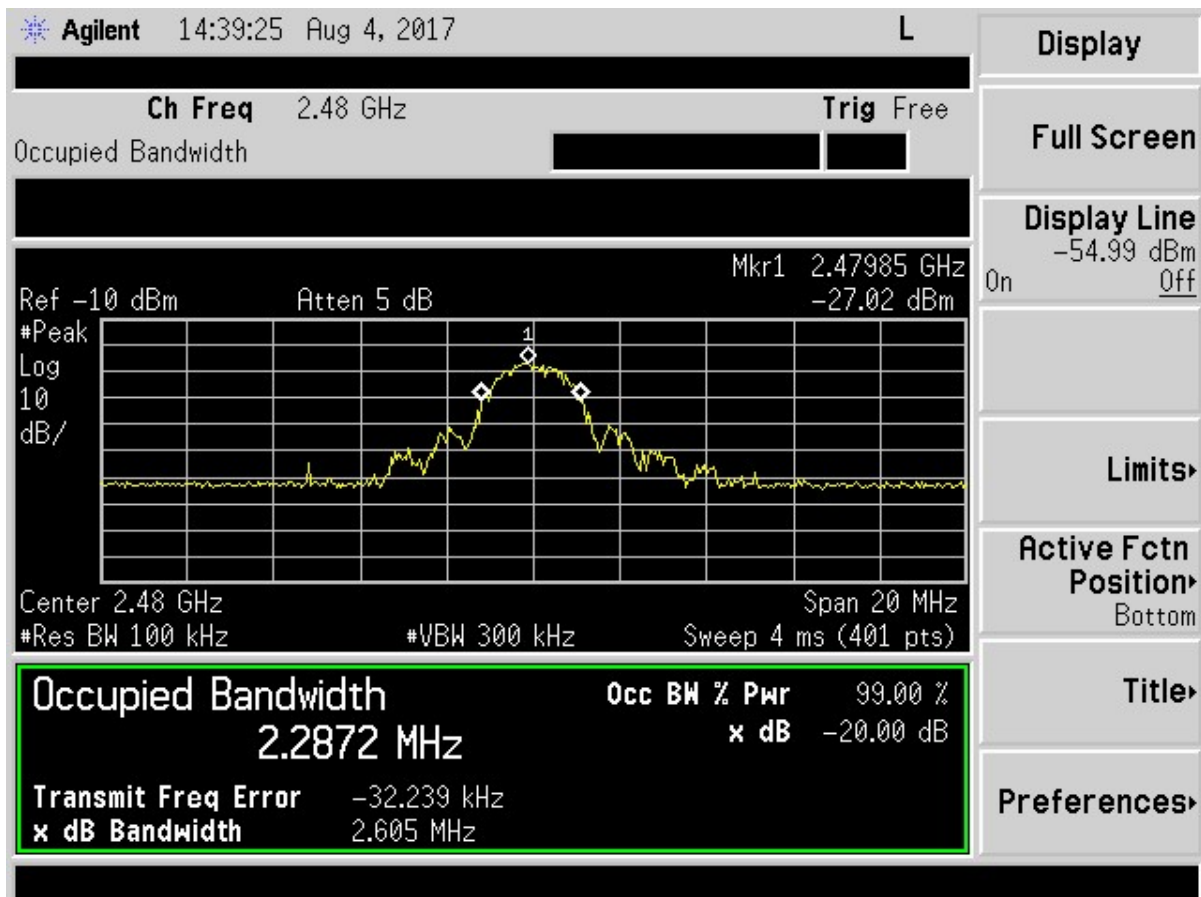
Figure 9. 99% Bandwidth – High Channel
