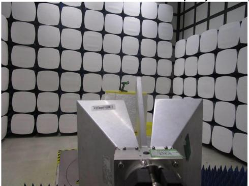
1.3 Radiated Emissions Test Setup
