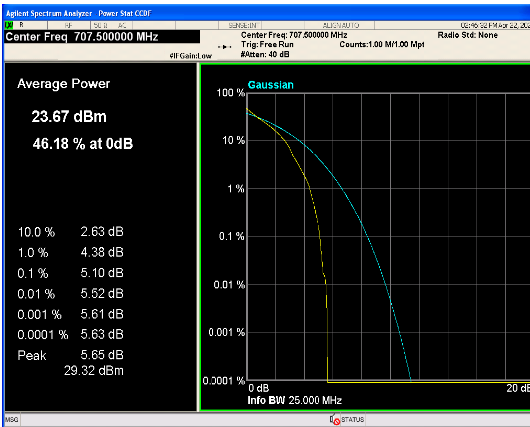
Band12 QPSK BW=5MHz Channel=23095 RB Size=1 Position=#0
