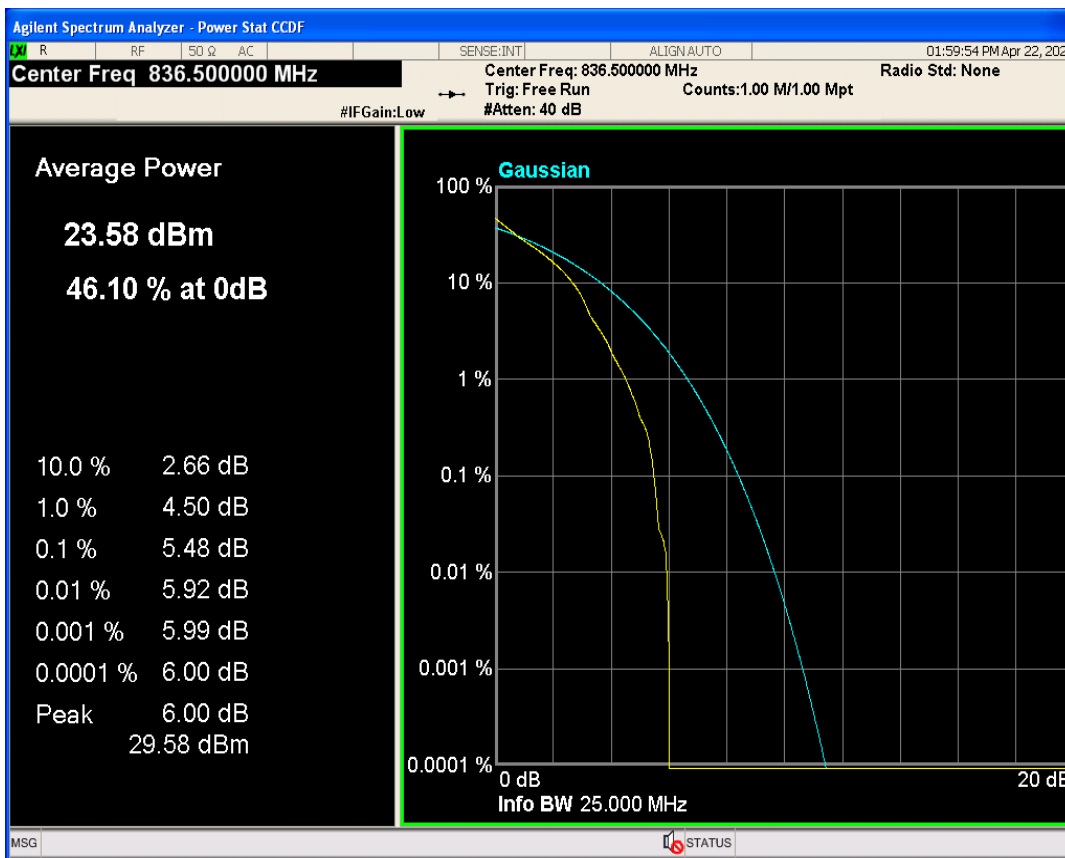
Band5 QPSK BW=5MHz Channel=20525 RB Size=1 Position=#0
