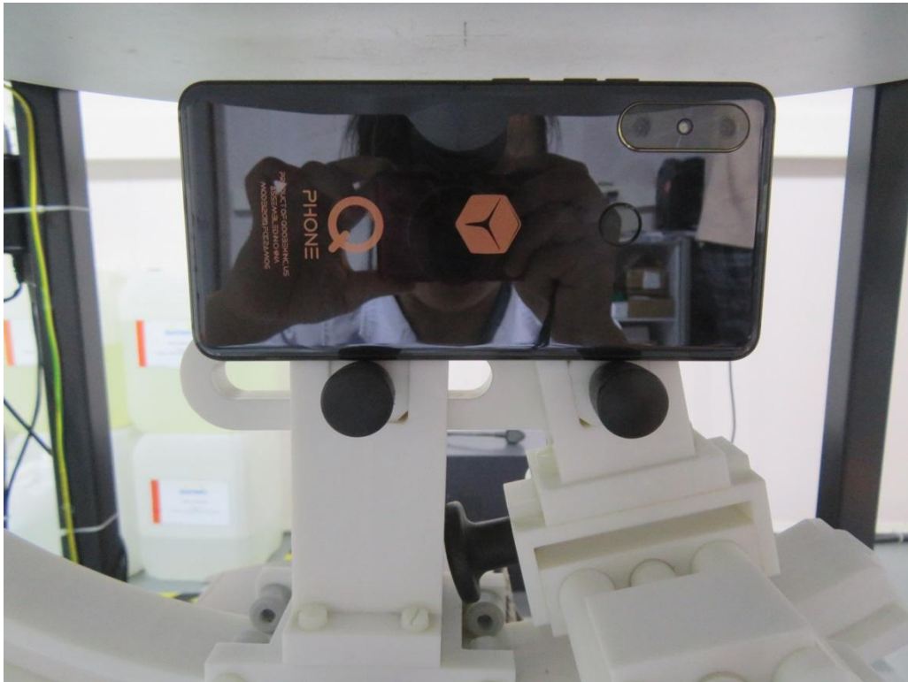
10mm body-worn Right Side Setup Photo (hotspot)
