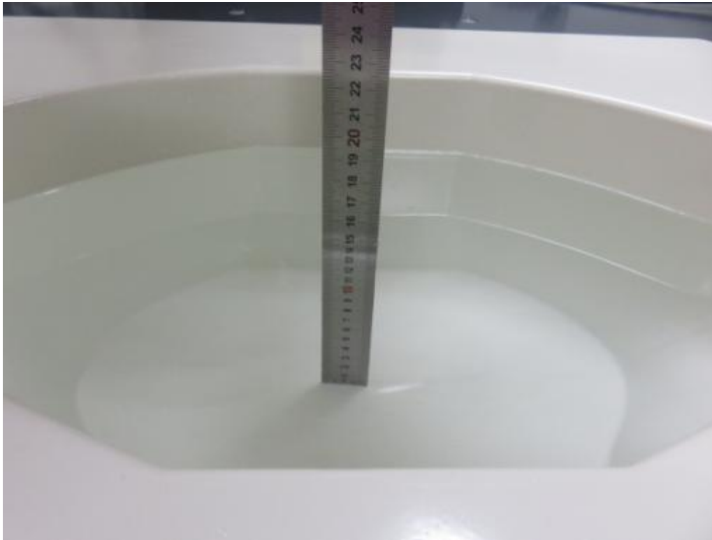
Photograph of the depth in the Body Phantom (835MHz, 16.0cm depth)
