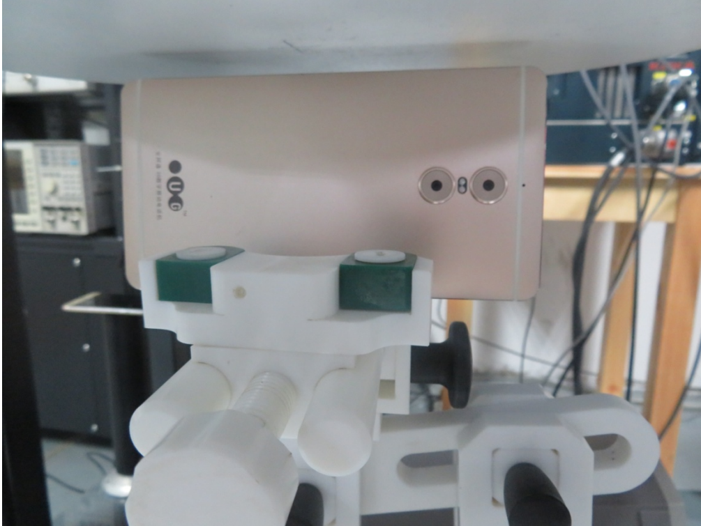
10mm body-worn Right Side Setup Photo (hotspot)
