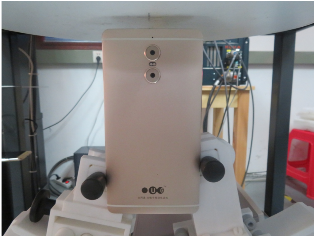
10mm body-worn Top Side Setup Photo (hotspot)
