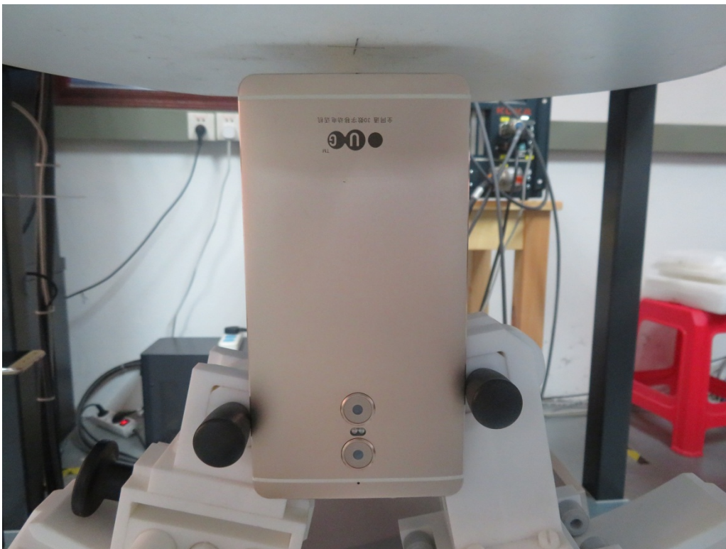
10mm body-worn Bottom Side Setup Photo (hotspot)
