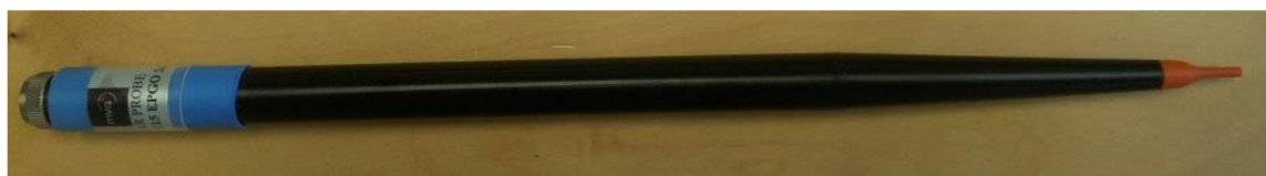
Figure 1 – MVG COMOSAR Dosimetric E field Dipole
