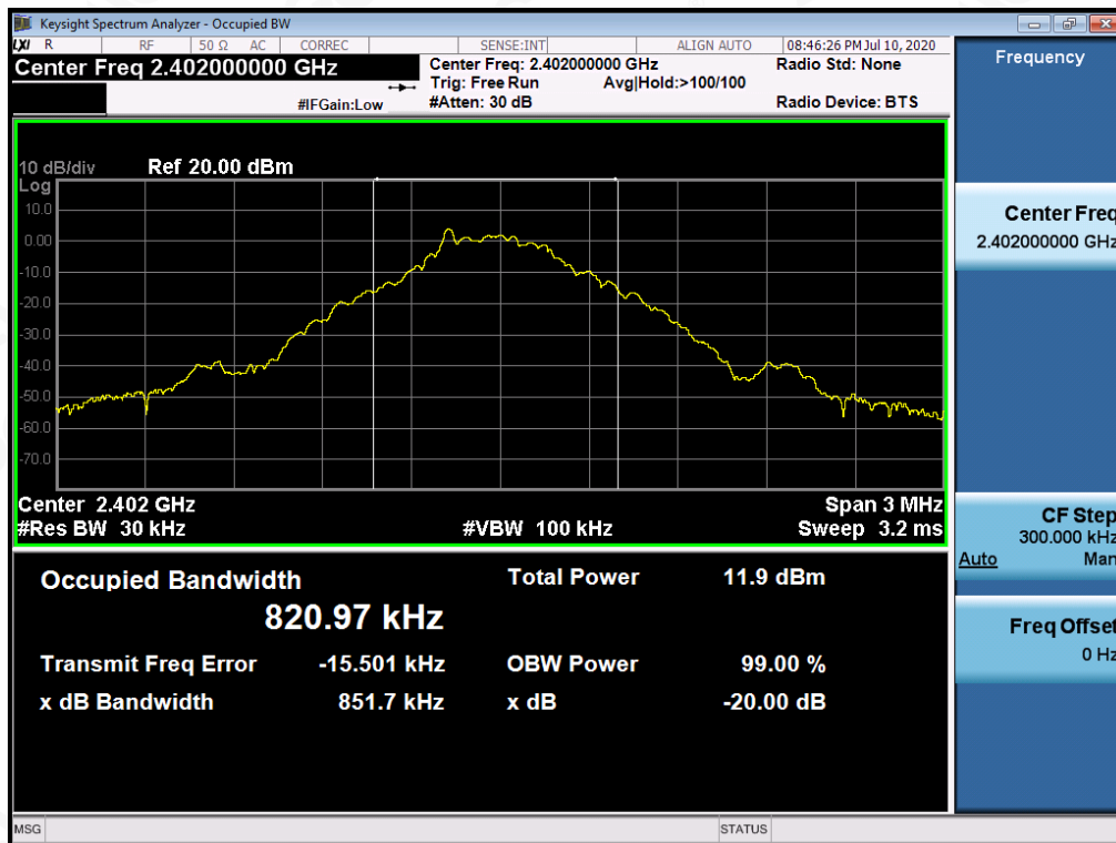
TEST PLOT OF BANDWIDTH FOR LOW CHANNEL
