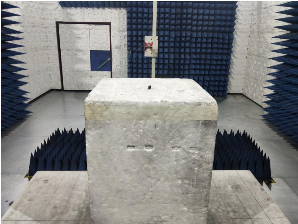
RADIATED EMISSION TEST SETUP ABOVE 1GHZ
