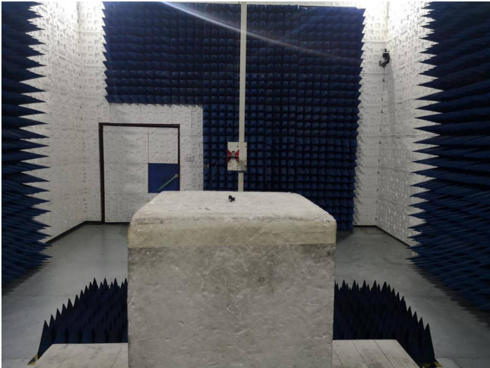
RADIATED EMISSION TEST SETUP ABOVE 1GHZ
