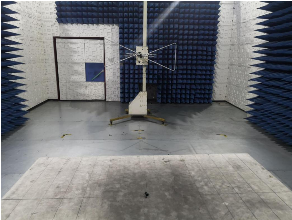
RADIATED EMISSION TEST SETUP ABOVE 1GHZ
