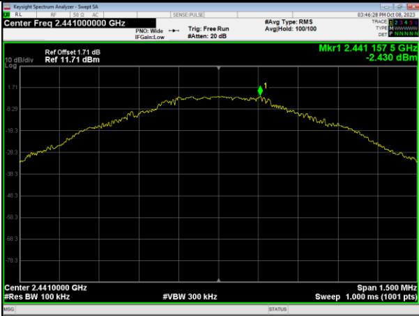
GFSK on Channel 39
