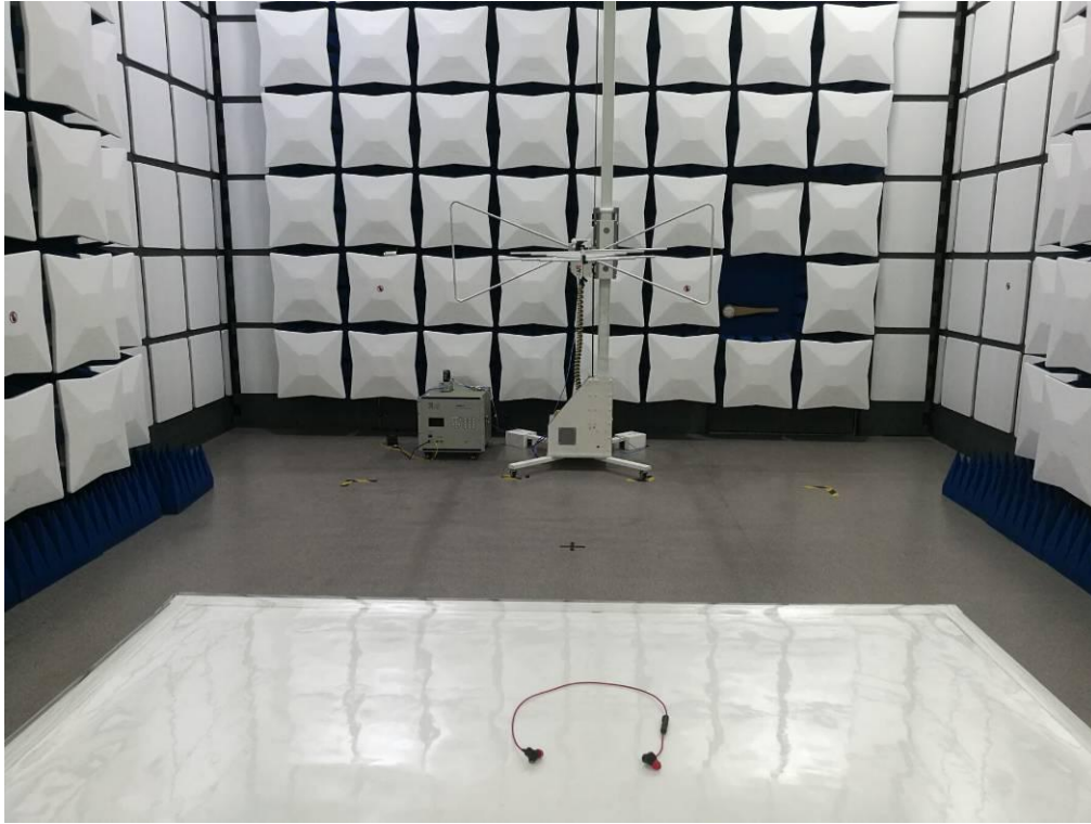
FCC RADIATED EMISSION TEST SETUP
