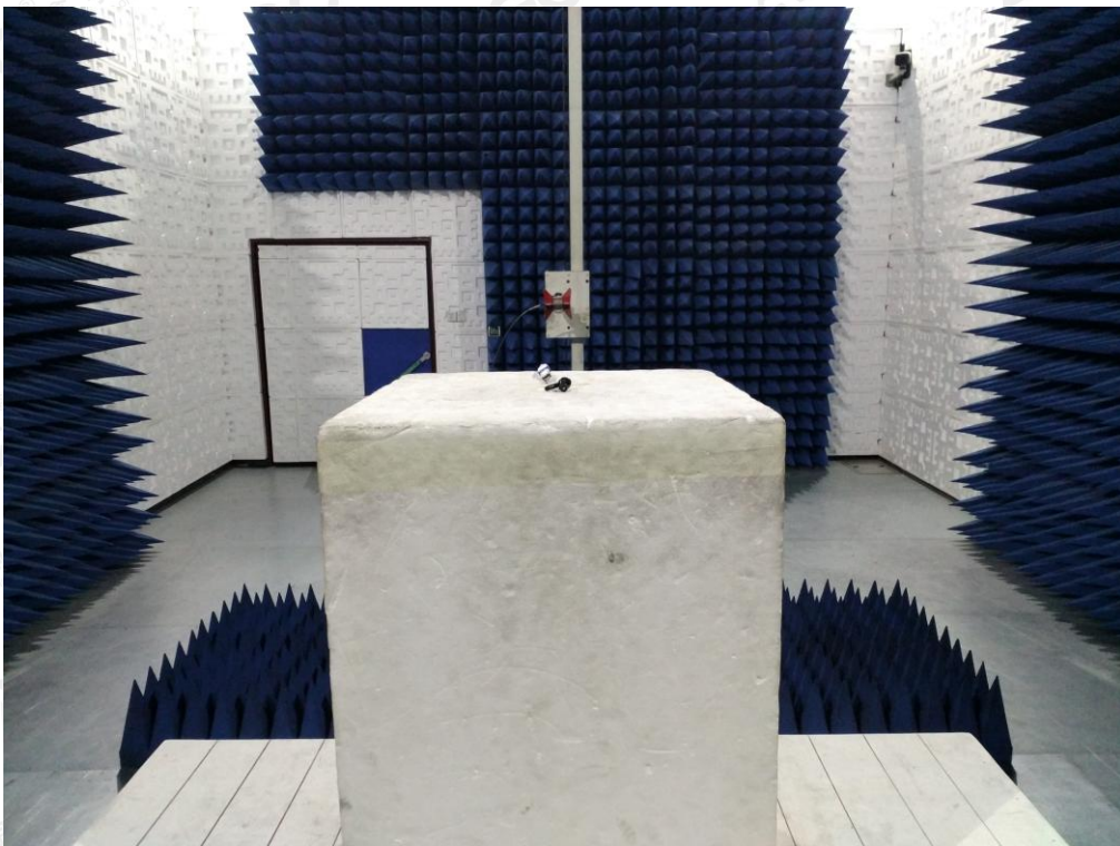
RADIATED EMISSION TEST SETUP ABOVE 1GHZ
