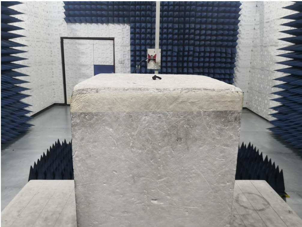
RADIATED EMISSION TEST SETUP ABOVE 1GHZ
