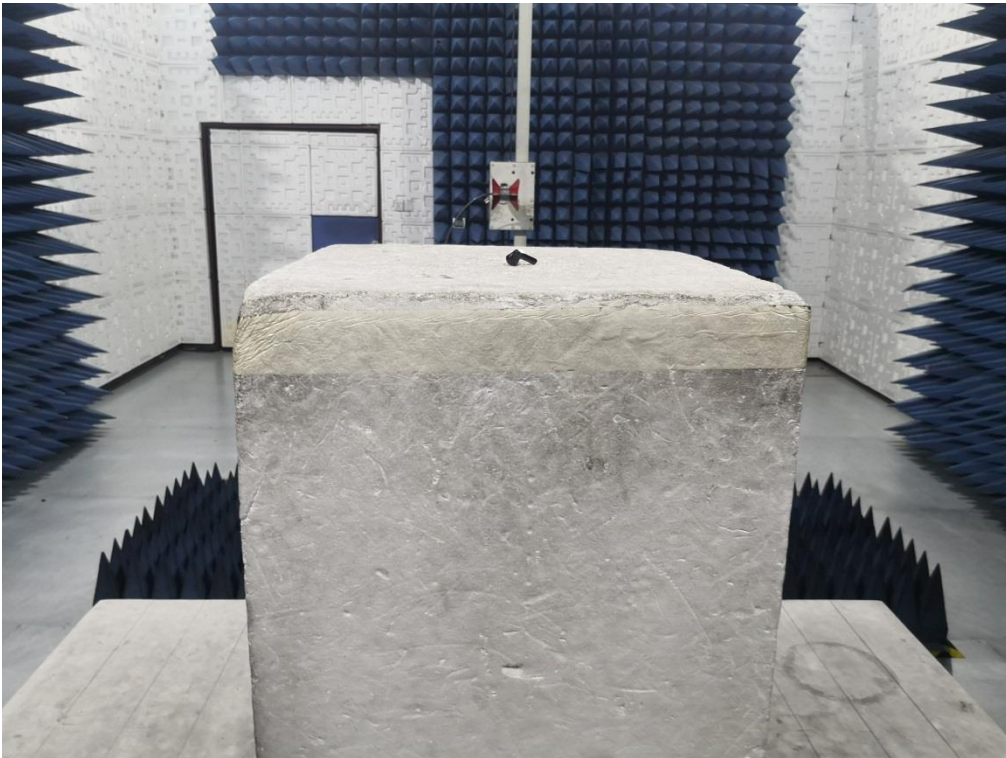
RADIATED EMISSION TEST SETUP ABOVE 1GHz
