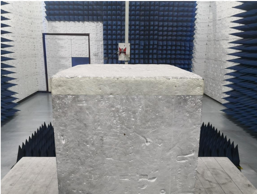
RADIATED EMISSION TEST SETUP ABOVE 1GHZ
