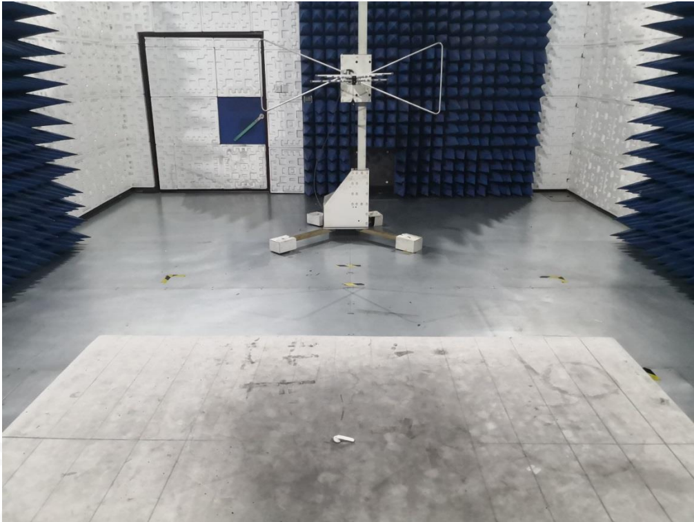
RADIATED EMISSION TEST SETUP ABOVE 1GHZ
