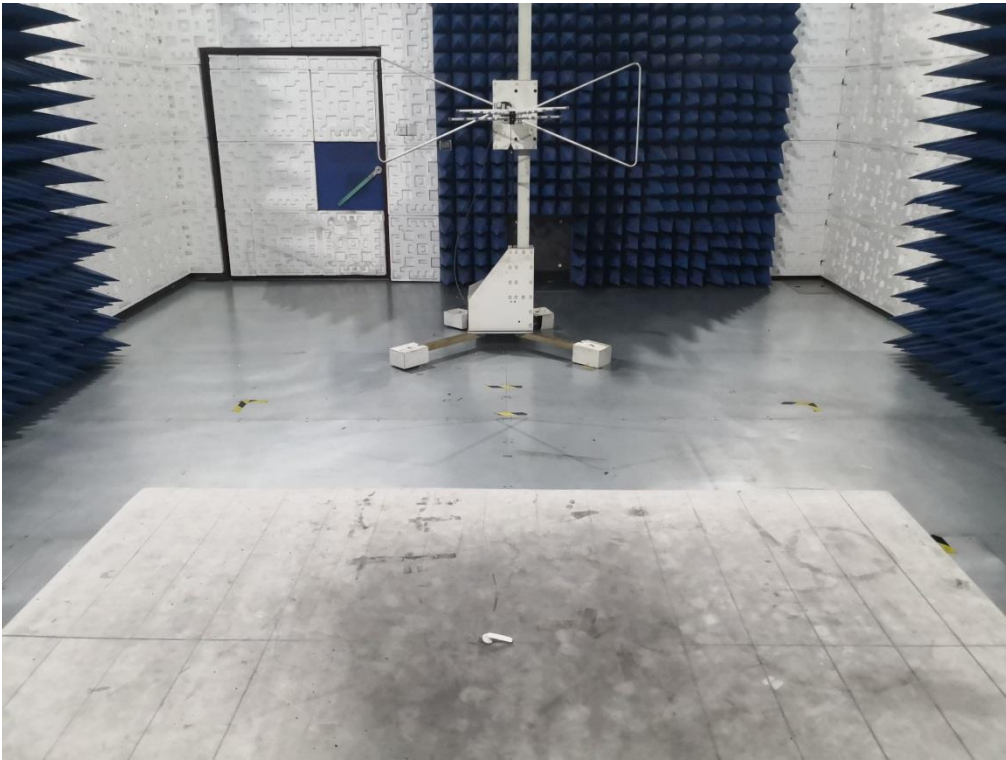
RADIATED EMISSION TEST SETUP ABOVE 1GHz
