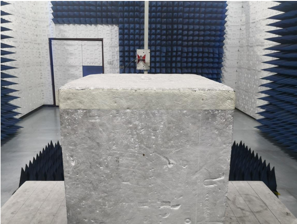
RADIATED EMISSION TEST SETUP ABOVE 1GHz
