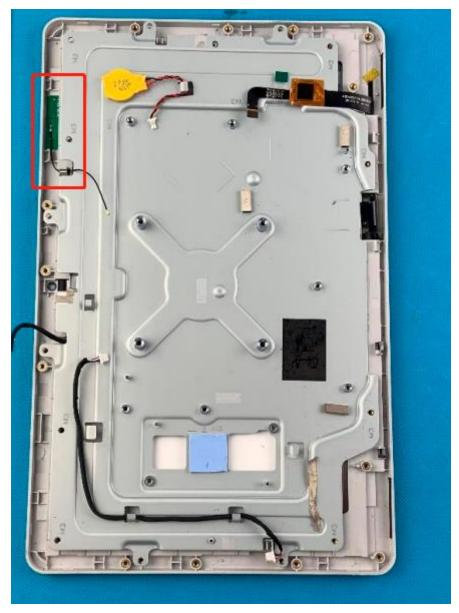
Note: The product uses internal antenna, which meets the requirements of FCC 15.203.
