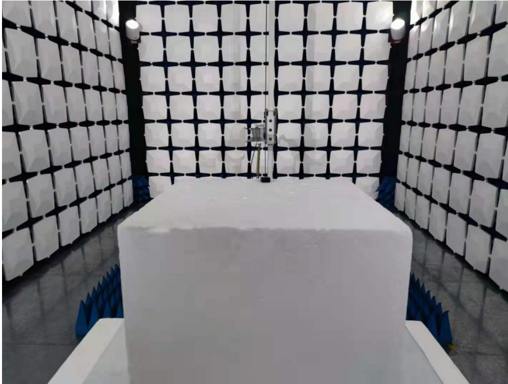
Above 1GHz for radiated emission test setup
