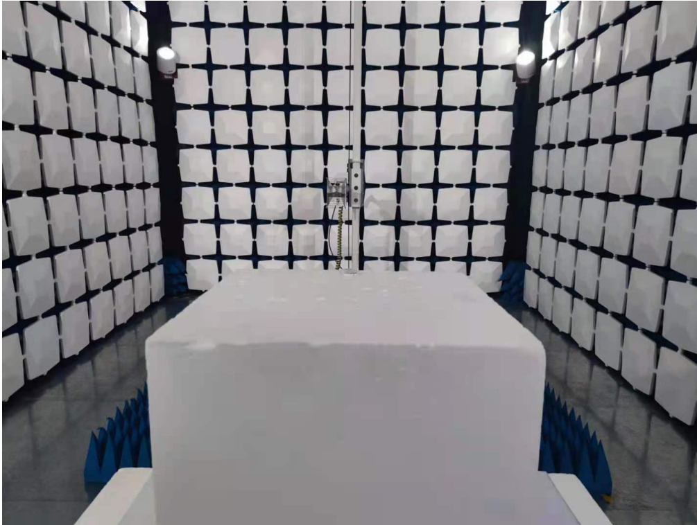
Above 1GHz for radiated emission test setup
