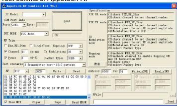
The test softeware was used to control EUT work in continuous TX mode, and select test channel, Wireless mode as below table
