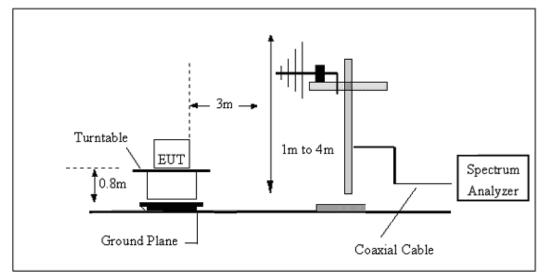
(C) Radiated Emission Test-Up Frequency Above 1GHz
