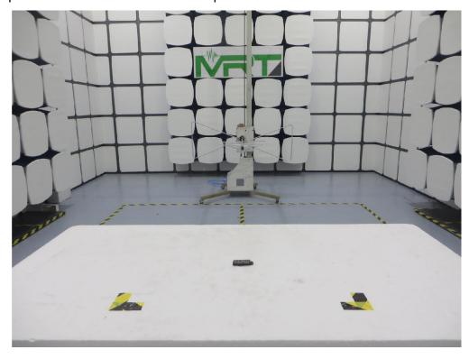
Description: Radiated Emission Test Setup for above1GHz
