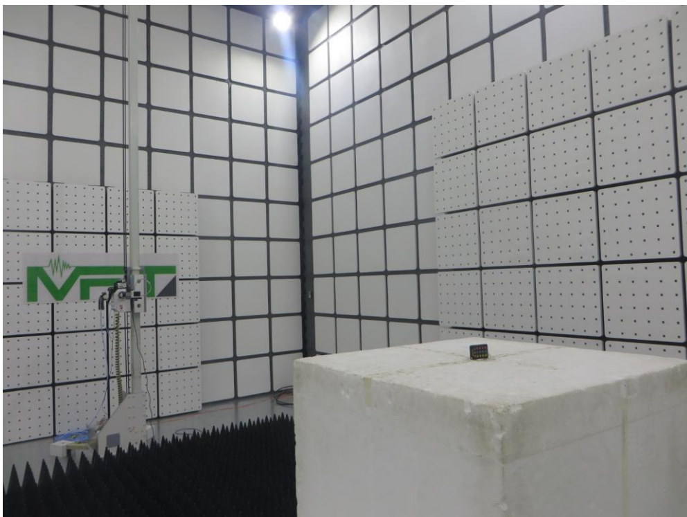
Description: Radiated Emission Test Setup for 18G ~ 40GHz
