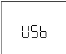
*LCD displays "USB" when logger connected to PC.*
