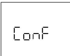
*LCD displays "CONF" for configuration success when connection with PC remains. (Only applicable to non-software configuration).*
