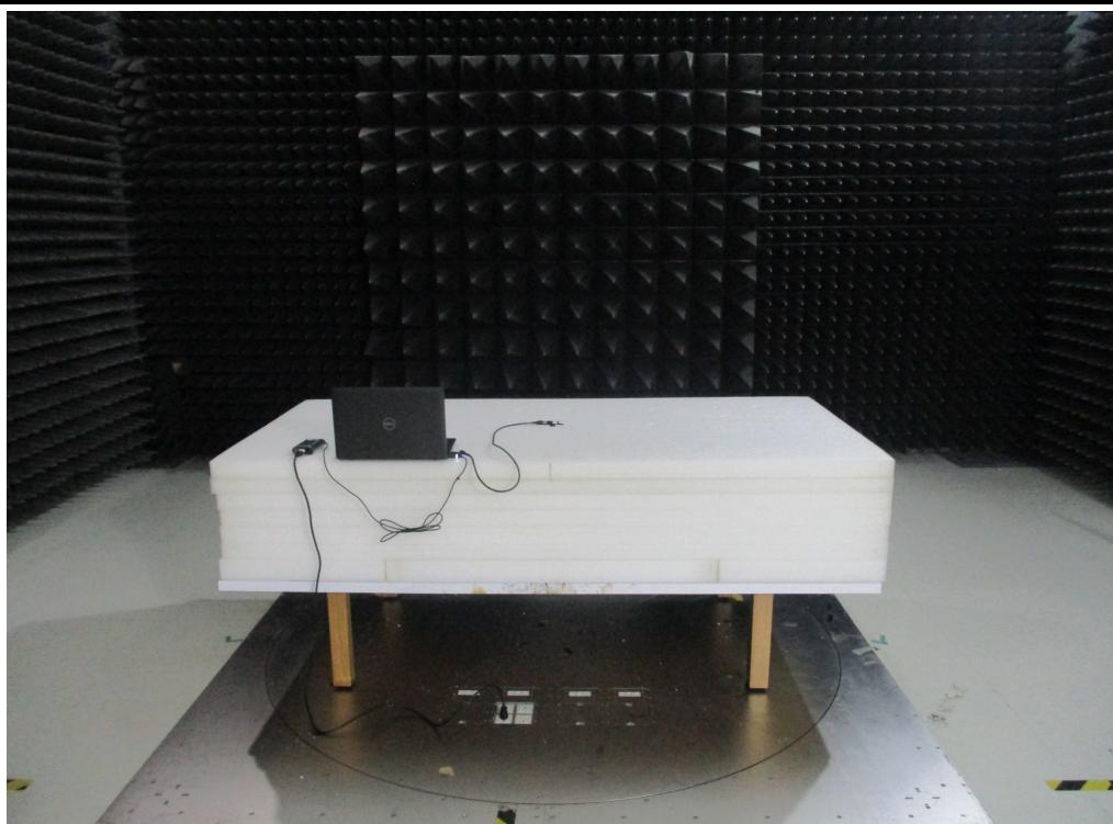
**Radiated Emission Below 1GHz Test**
