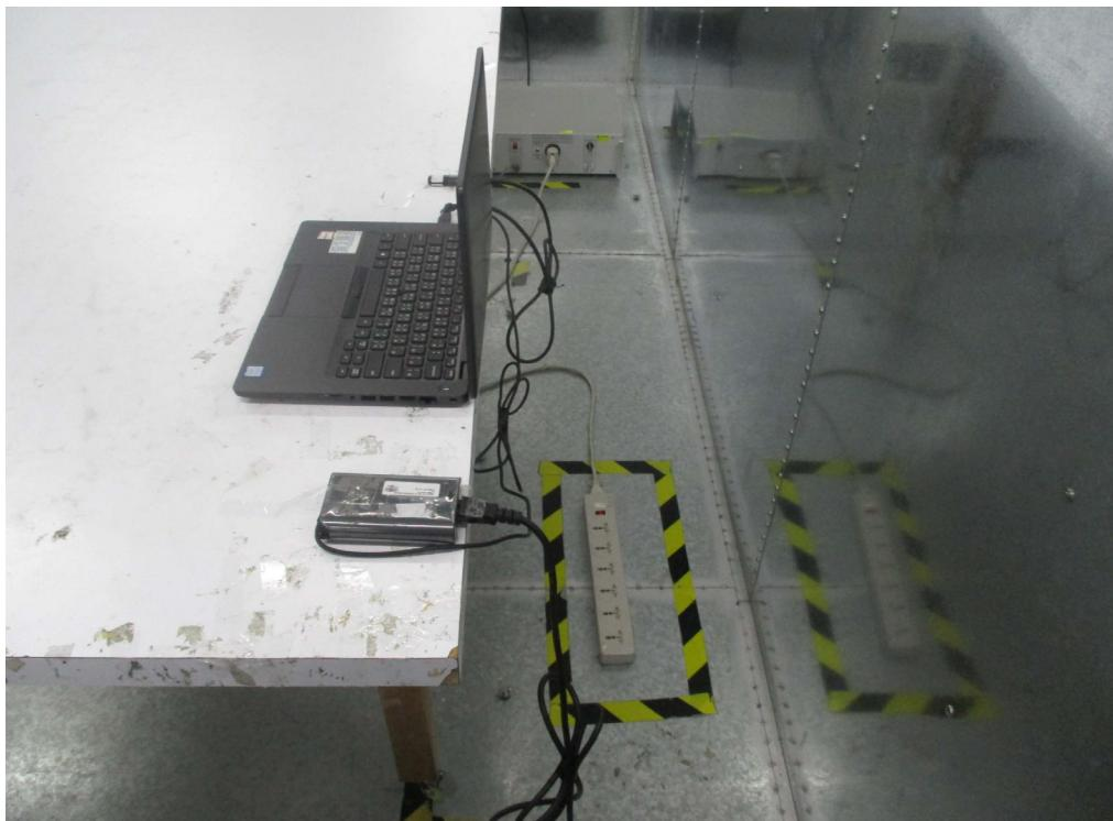
**Radiated Emission Below 1GHz Test**
