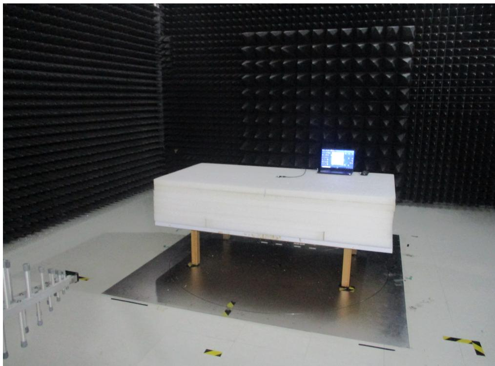
**Radiated Emission Above 1GHz Test**
