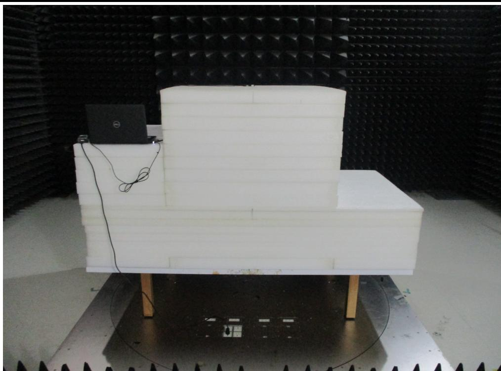
**Radiated Emission Above 1GHz Test**
