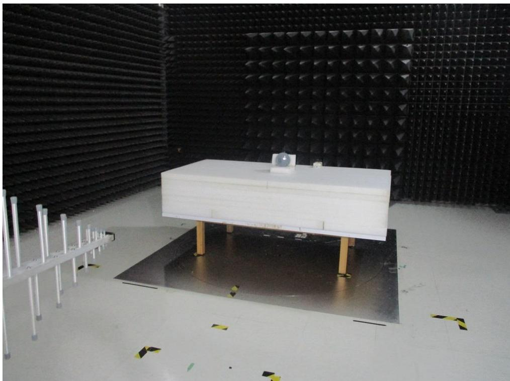
**Radiated Emission Above 1GHz Test**
