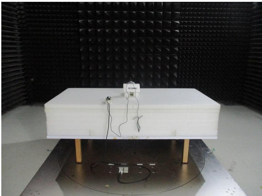
**Radiated Emission Below 1GHz Test**
