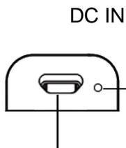
The indicator turns red under charging and turns off when the speaker is fully charged. The fully charged speaker can work around 3 hours. Low battery leads to alarm or auto stopped. Please charge the speaker in time.
