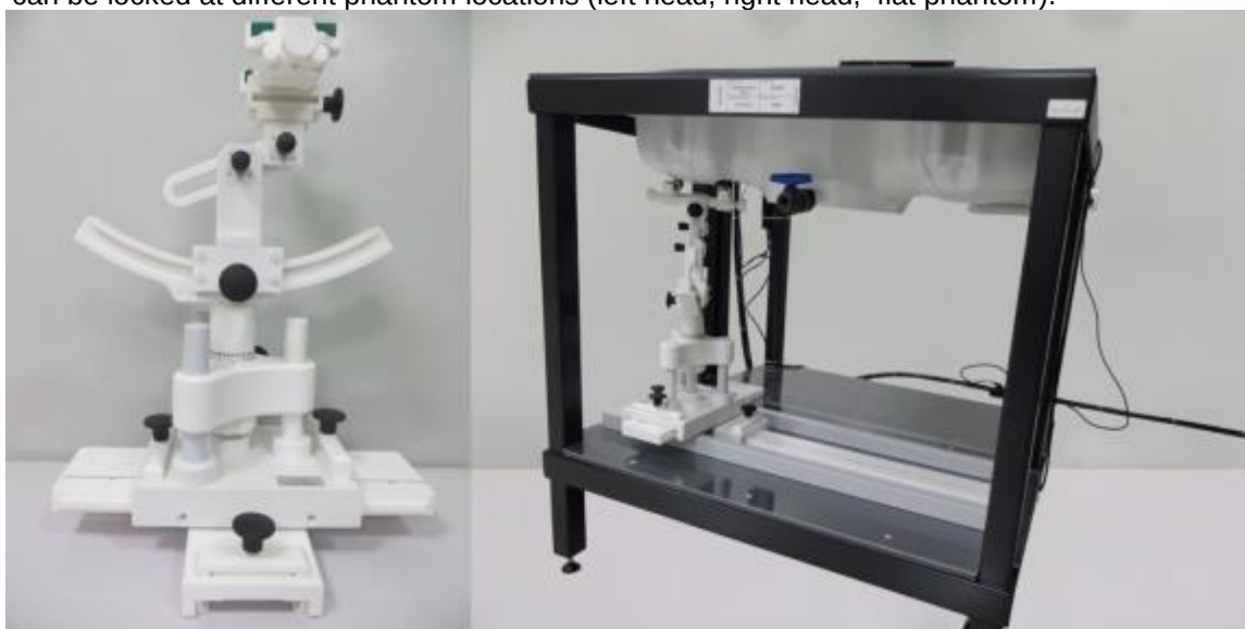
Device holder supplied by SATIMO
