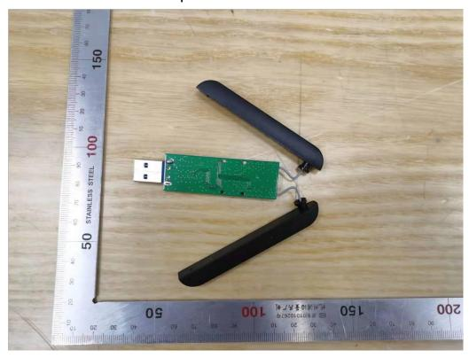
Note: The two antennas are soldered on the PCB board.
