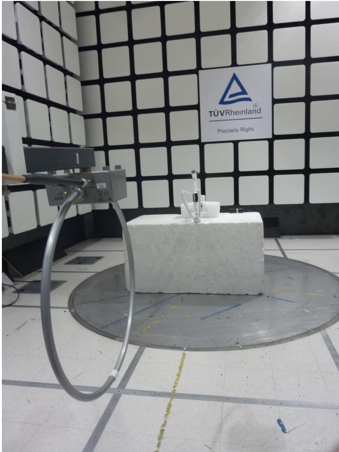
Figure 1: Test Setup for Radiated Emissions 9 kHz to 30 MHz
