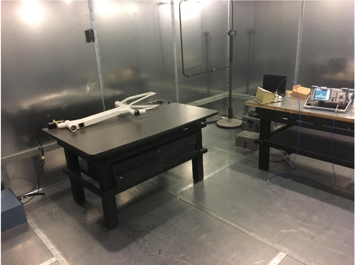
Figure 5: Test Setup for AC Line Conducted Emissions
