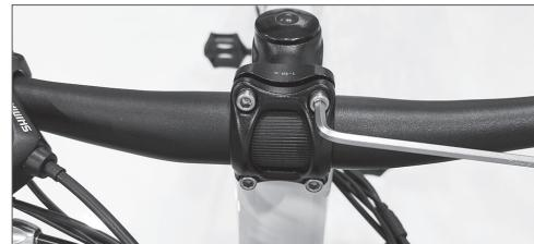
4. Assemble and center the stem so the handlebar is perpendicularly aligned with the front wheel. Tighten the (2x) 5mm hex screws on the stem to 8Nm - 9Nm of torque.
