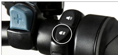
This will turn on the front headlight. To turn off the main headlight hold down the headlight button for 2-3 seconds.
