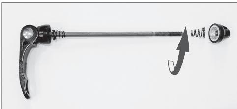
2. Assemble the front wheel on the bike's front fork.
