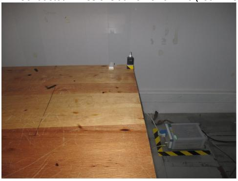
1.2 Radiated Emissions Test Setup
