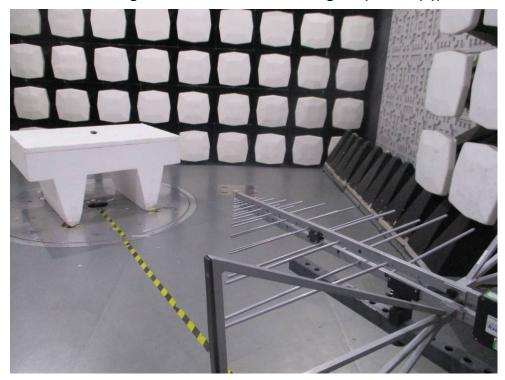
1.2 Radiated Emissions Test Setup (below 1GHz)
