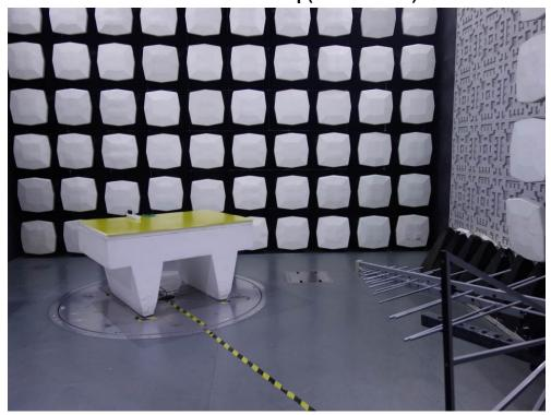
1.4 Radiated Emissions Test Setup(above 1GHz)
