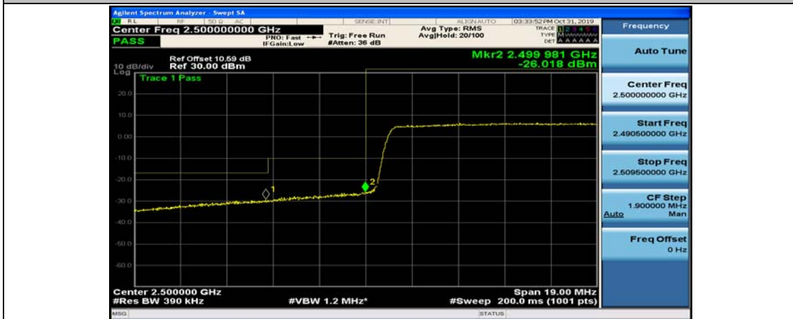
(Channel Bandwidth:20 MHz)_LCH_16QAM_100RB#0
