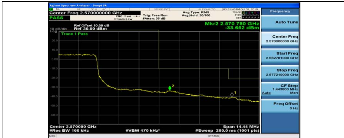
(Channel Bandwidth:15 MHz)_HCH_16QAM_37RB#38
