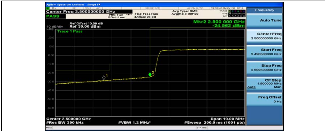
(Channel Bandwidth:20 MHz)_HCH_QPSK_1RB#0
