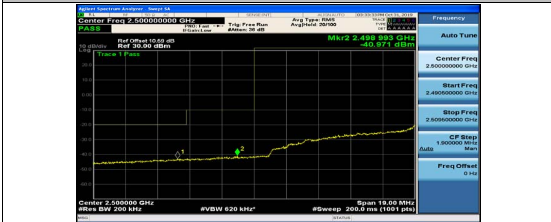
(Channel Bandwidth:20 MHz)_LCH_16QAM_100RB#0
