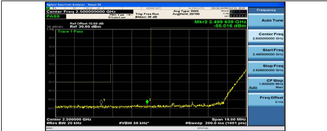
(Channel Bandwidth:20 MHz)_LCH_16QAM_1RB#99
